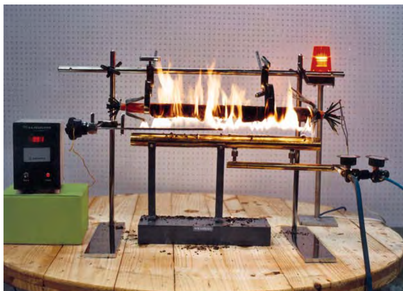
3 Hours fire survival test as per IEC-331
