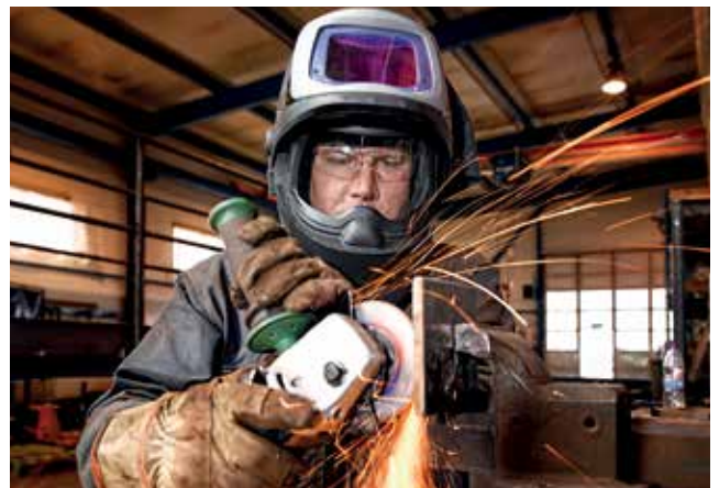
As additional head and neck coverage there are flame-retardant accessories for protection of molten metal, sparks and flames.
