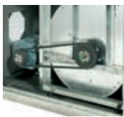
Motor outside the airflow path
