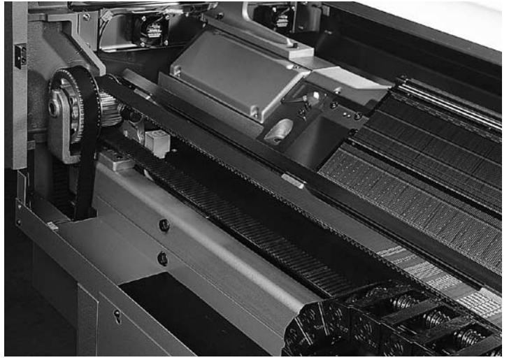
Large Knitting Machine (SUPER TORQUE Timing Belt)
