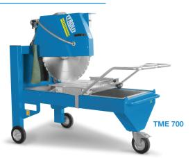
Maximum stability and robustness due to torsional steel chassis. Removable water tank for easier cleaning. Sturdy, balanced transport hook for easy crane transport. Precise mitre cutting thanks to mitre stop.
